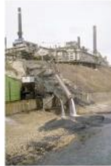
Figure 3.11 Point sources of pollution, such as this factory's waste water, are easier to identify than non-point sources.
